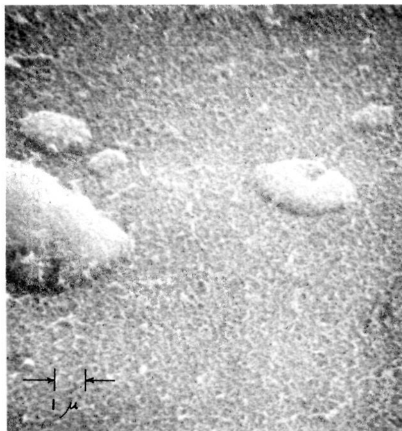
Figure 2. Scanning electron microgram of the glass bead surface coated with cellulose nitrate membrane, \times 2600 .
